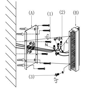
To prevent moisture from entering the outlet box and causing a short, seal around the top and side perimeter between the fixture and the wall surface with weather resistant caulking (see illustration a). The space at bottom should be
